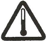
Hot surface warning
